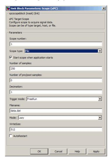
5 Select the Start scope when application starts check box to start a scope when the target application is downloaded and started. The scope window opens automatically.
