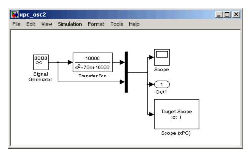
The Simulink block diagram opens for the model my\_xpc\_osc2.mdl.
