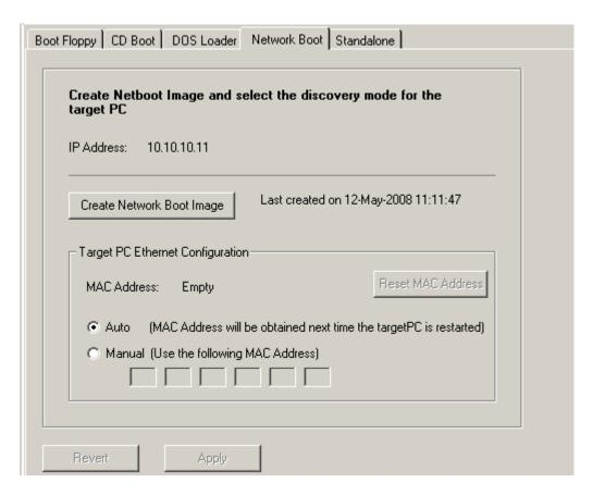
The **Target PC Ethernet Configuration** section of the configuration pane allows you to either associate a physical target PC MAC address with the xPC Target Explorer target PC name, or allow the software to automatically find target PC MAC addresses. If you want to associate your physical target PC MAC address,
