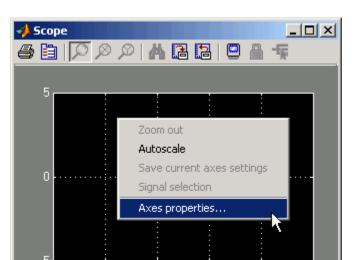
**5** In the Scope window, point to the *y*-axis shown in the figure below, and right-click.
