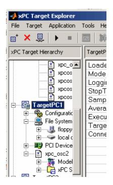
Alternatively, you can now drag a prebuilt target application, DLM, to a target PC icon. If a connection does not already exist, xPC Target Explorer optionally creates a connection to that target PC.
