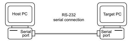
For detailed information on setting up the hardware and software for serial communication, see "Serial Communication" on page 2-37.
